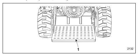
Figure 3-7 Operator's Platform and Safety Treadle
